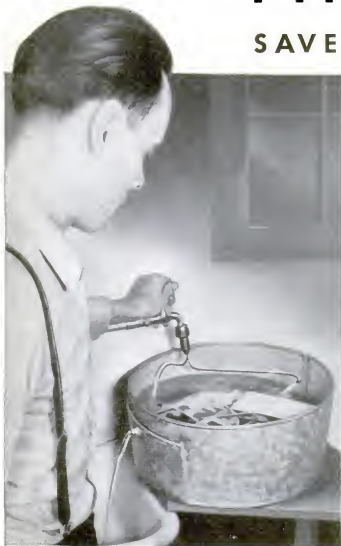
The prints are washed quickly by a whirling motion, and the hypo-laden water is drained from the bottom
